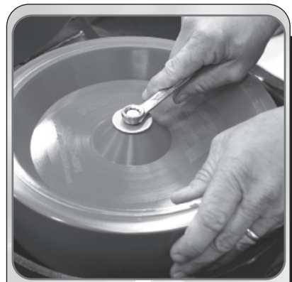
Figure 8 Hold wheel in place while loosening bolts.
